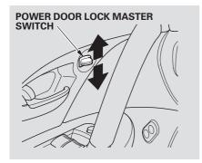
Each front door has a power door lock master switch. Either switch locks and unlocks all doors. Push the switch down to lock all doors and up to unlock them.
