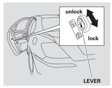
The childproof door locks are designed to prevent children seated in the rear from accidentally opening the rear doors. Each rear door has a lock lever near the edge. With the lever in the LOCK position, the door cannot be opened from the inside regardless of the position of the lock tab. To open the door, push the lock tab in, and use the outside door handle.
